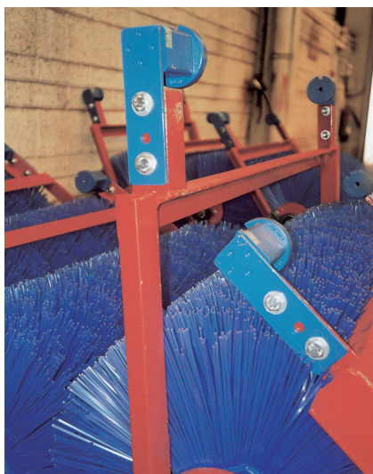
Suspension of circular brush on potato harvester
