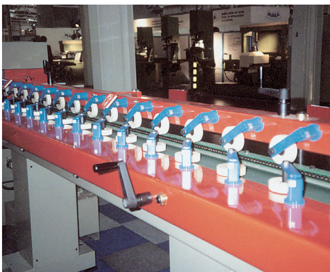
Suspension of tensioning rollers on milling machine in the wood industry
