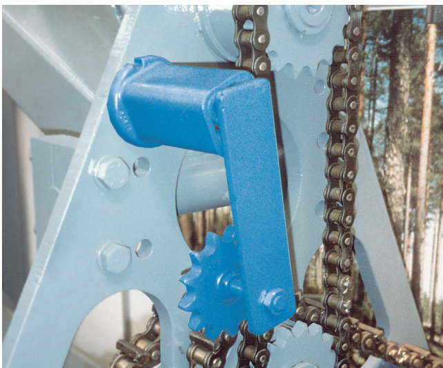
Chain tensioner on paper rolling mechanism
