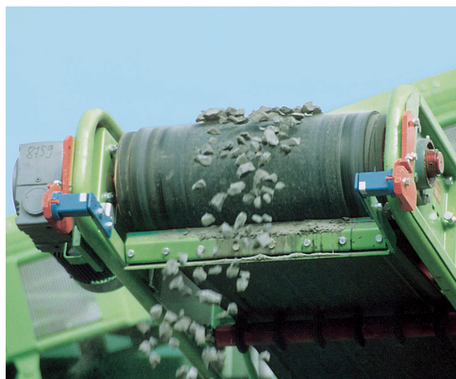
Elastic suspension on belt scraper
