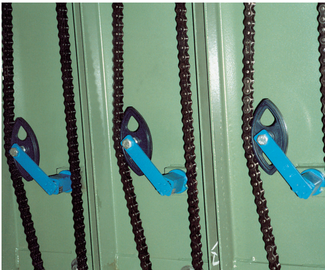
Chain tensioner with glider on processing machine
