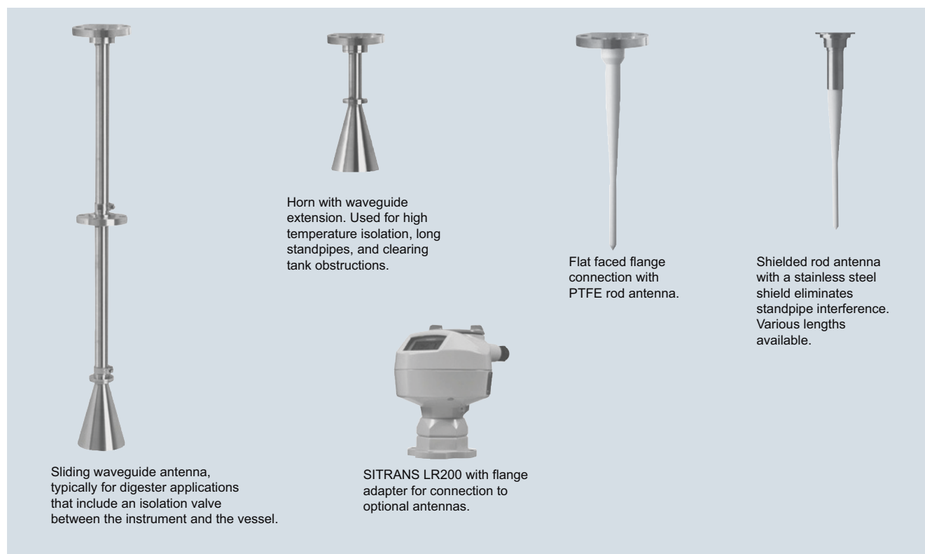
Antenna configurations for SITRANS LR200
