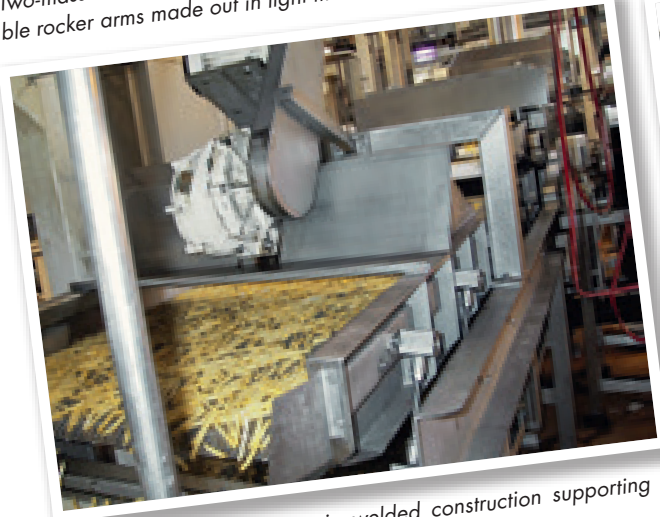
One mass shaker conveyor with built-in screening fraction for the transport and sorting of wood-chips
