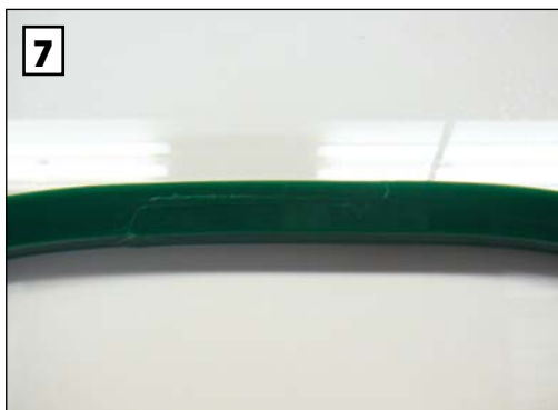
7 Remove the belt and clean the welding point.
