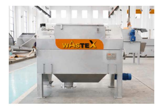
IRDS internally fed rotary drum screen is the equipment for medium flow, medium low solid rate wastewater. It is compact sized, completely closed and low malfunction machine, which is solid-liquid separation device for normal wastewater. The cuneal or punched type filter can be choose with the machine, the most common aperture is 0.25~6mm.
